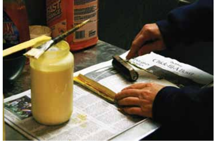
When gluing sheets of paper together to form turning blocks, flatten the individual sheets using a roller. This process expels air pockets.
