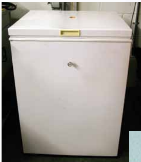
The artist’s dryer is a converted chest freezer. A 100-watt lightbulb on the inside helps maintain 155°. A hole in the top and two in the bottom allow airflow.
